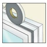
The sealing tape can advantageously be mounted immediately prior to window installation.
